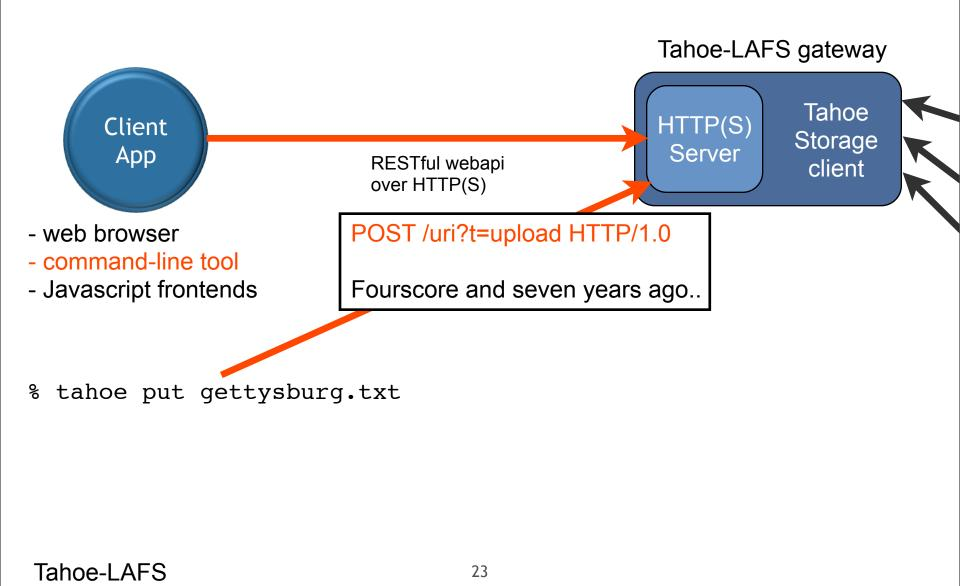
The most basic operation is to upload a file into the grid through the CLI "put" command. This simply takes the input data and sends it in the body of an HTTP "POST" to a special URL hosted in the gateway process.
