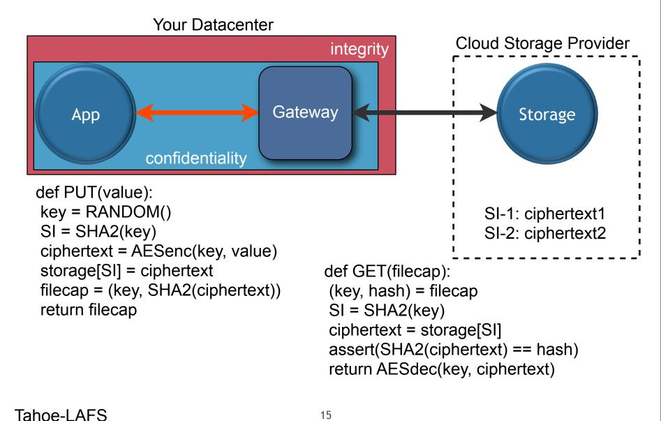
We can protect our data's integrity against errors in the storage system by hashing the ciphertext before delivery, and checking that hash upon retrieval. A hash failure is treated identically to a failed read: availability is lost, but integrity is uncompromised. This protects the application against undetected errors on the storage host.
