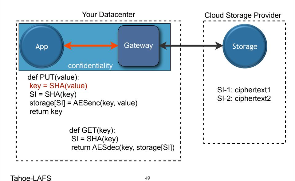
Optionally, we use another trick called "convergent encryption", in which the encryption key is a secure hash of the plaintext. This has the convenient property that uploading the same file twice results in the same ciphertext, which can be shared between the two instances to save space.
