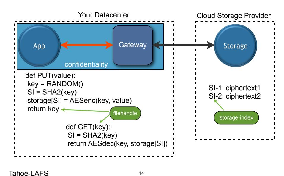
So our first step is to insert a gateway, which encrypts the data before giving it to the storage system. We generate a new unique AES key for each file, and return that key to the application as the filehandle. We derive a "storage index" from that key with a one-way hash, to tell the storage provider where to store the ciphertext. This saves us from needing to remember the storage index separately for each file.
